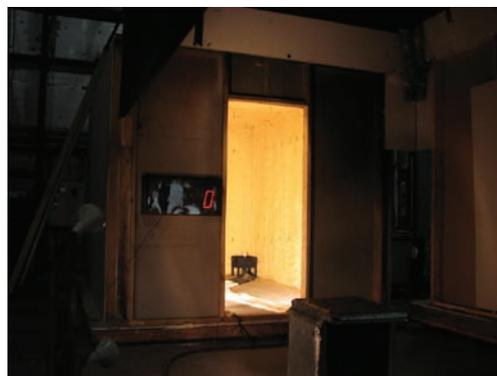
Figure 2. The NFPA 286 test assembly
