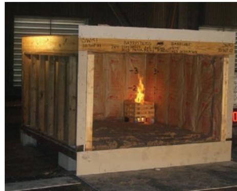
**Figure 1. The SwRI 99-02 comparative crawl space test showing a baseline assembly constructed with Kraft paper facing exposed to the flame source.**
